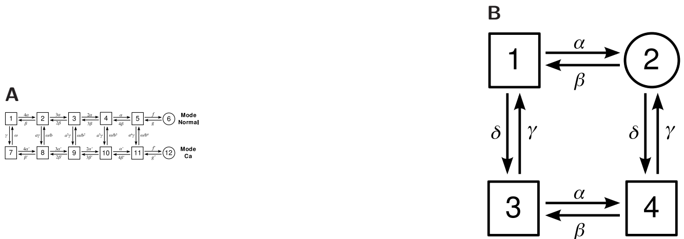
Figure 33.2: A : State diagram of the discrete LCC Markov model from [?]. Each channel can be in one of the 12 states. The transition between the states are controlled by propensities. The \alpha , and \beta are voltage dependent, \gamma is [Ca^{2+}] dependent and f , a , b , and \omega are constant, see [?] for further details. The channels operates in two modes: Mode normal , represented by the states in the upper row, and Mode Ca , represented the states in the lower row. In state 6 and 12 the channel is open, but state 12 is rarely entered as f' \ll f , effectively making Mode Ca an inactivated mode. B : State diagram of a RyR from [?]. The \alpha and \gamma propensities are Ca^{2+} dependent, representing the activation and inactivation dependency of the cytosolic [Ca^{2+}] . The \beta and \delta propensities are constant.
