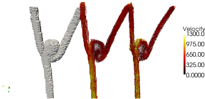
Figure 23.12: Figure showing resolution of data points where velocity measurements are made (left), velocity measurements from 4D PC MRA (middle), and CFD simulations (right).
