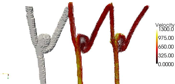
Figure 27.12: Figure showing resolution of data points where velocity measurements are made (left), velocity measurements from 4D PC MRA (middle), and CFD simulations (right).
