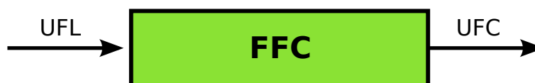
Figure 11.1: The form compiler FFC generates C++ code in UFC format from a given finite element variational form in UFL format.
