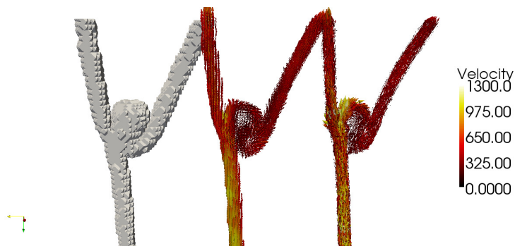
Figure 28.12: Figure showing resolution of data points where velocity measurements are made (left), velocity measurements from 4D PC MRA (middle), and CFD simulations (right).
