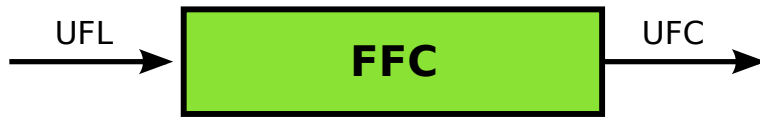
Figure 12.1: The form compiler FFC generates C++ code in UFC format from a given finite element variational form in UFL format.
